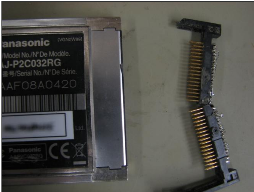
Figure B2: Header pins removed from one P2 card
