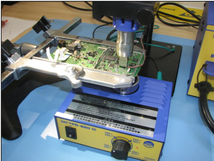
Figure A8: FBGA chip removal
