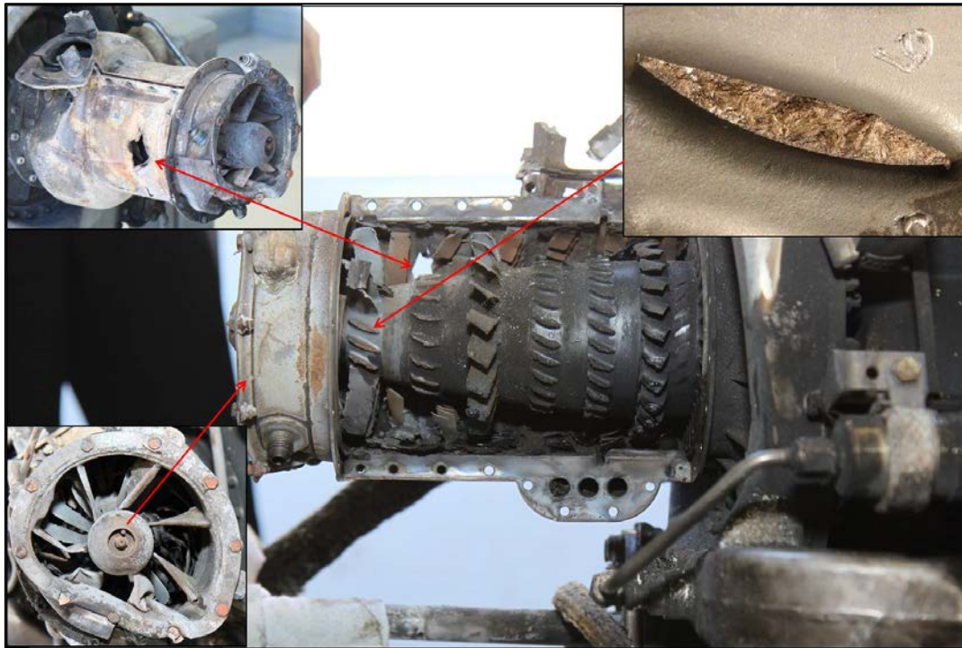
Figure C1: Left engine rotor pack with hole in casing and typical stage 1 blade overload failure
