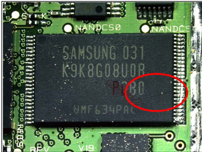
Figure A4: Location of damage to TSOP chip
