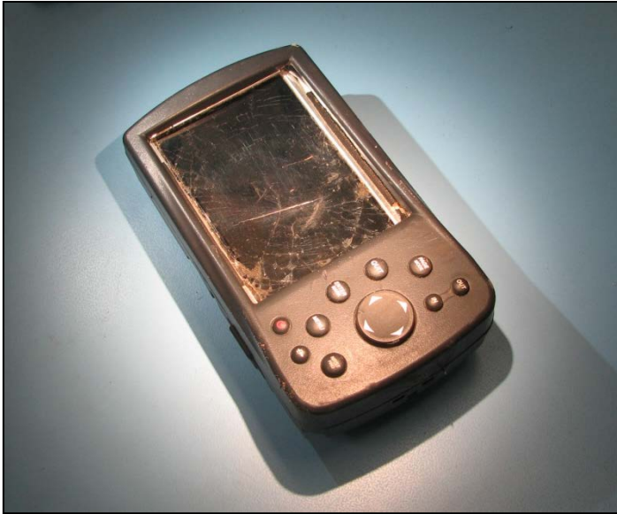
Figure A2: Recovered VH-NTV Garmin GPSMAP 495
